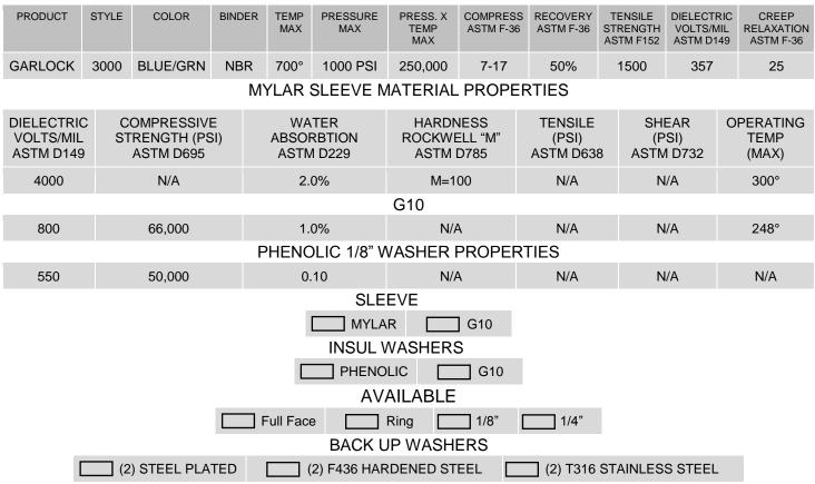
Note: 1/4 gaskets consist of 2-1/8" thick gaskets laminated at the factory.
