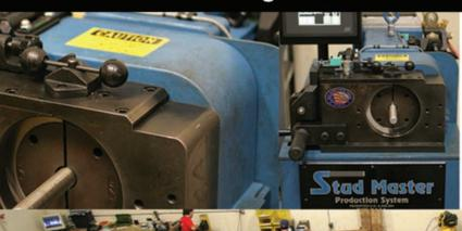
The Stud Master chamfering operation allows our staff to chamfer and mark as fast as they can load the machine. This machine also improves quality with precise and uniform chamfers as well as marking both ends of the material.
