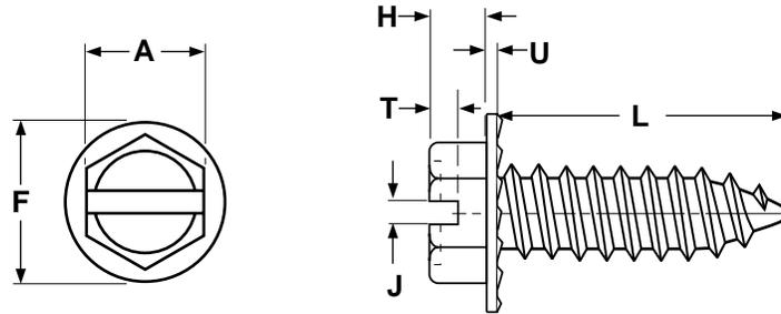
**SERRATED HEX WASHER SELF TAPPING SCREWS - TYPE-AB**
